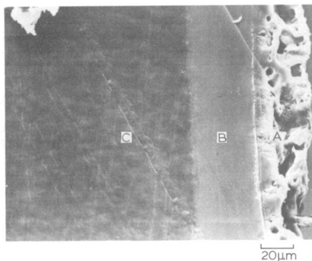
Figure 4 Cross-section of nylon-6 showing outer porous region (A), salt laden region (B) and unswollen core (C). Magnification 630× (Published by courtesy of J. Mater. Sci. (1979, 14, 2881))
